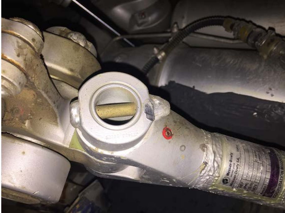
Incorrectly installed collar which shows evidence of contact with link unit
