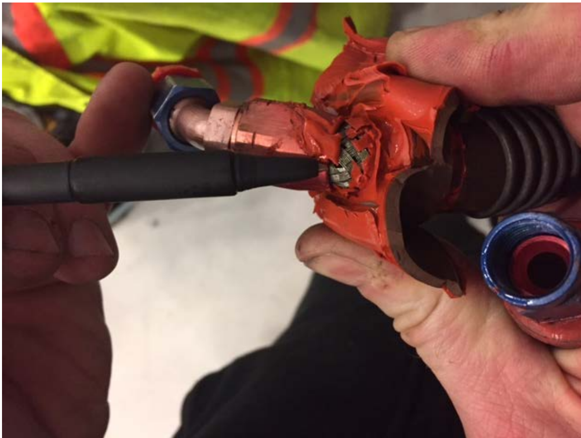
Leak in a braided fuel line
