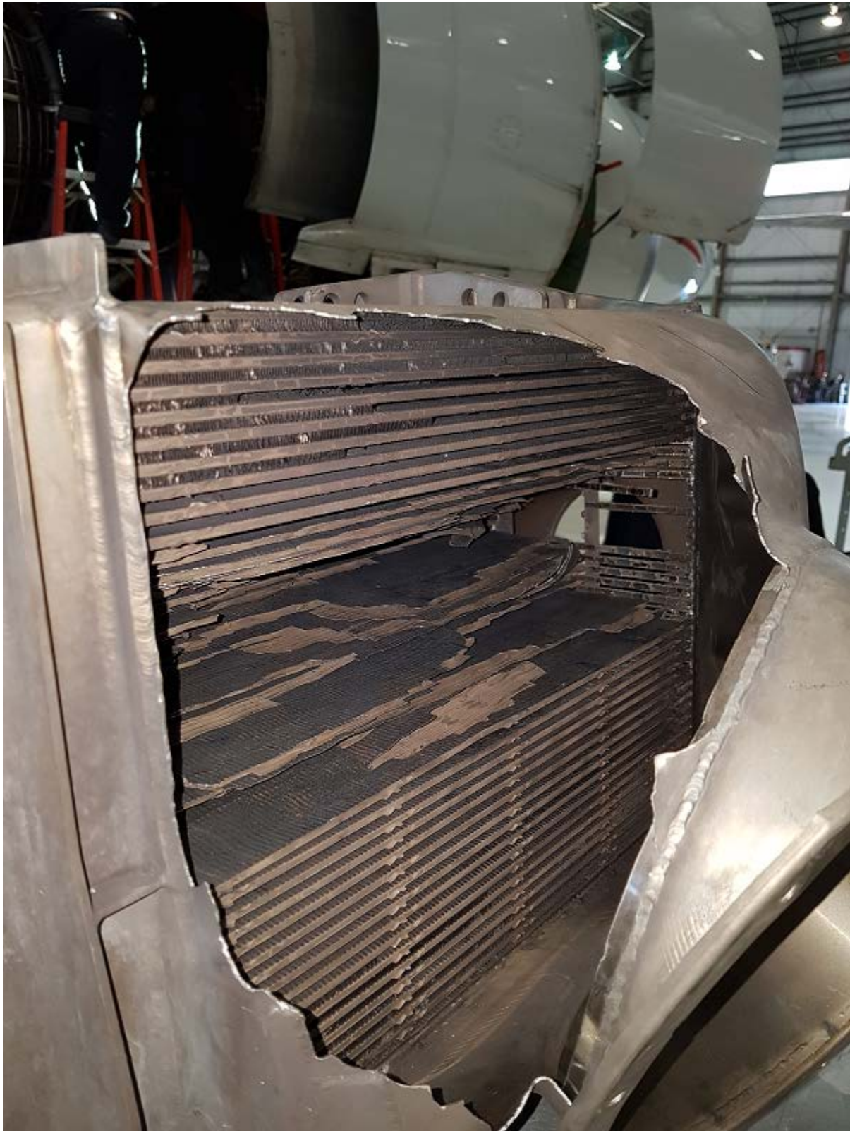
Close up view of the hole in the housing and missing fins on the internal structure.
