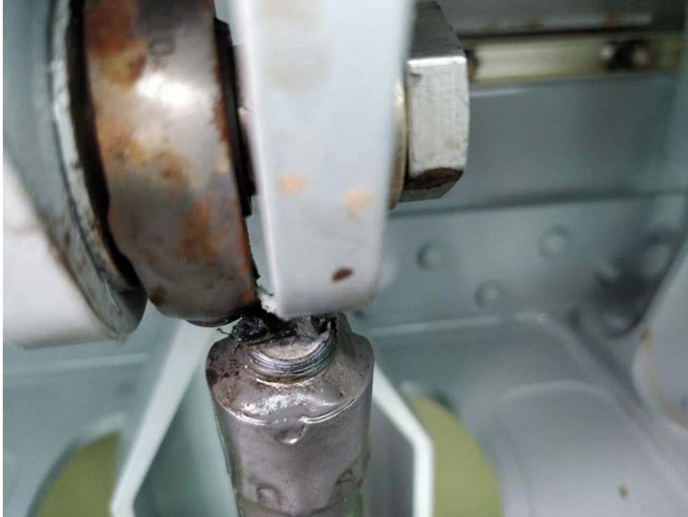
Sheared rod end with visible corrosion
