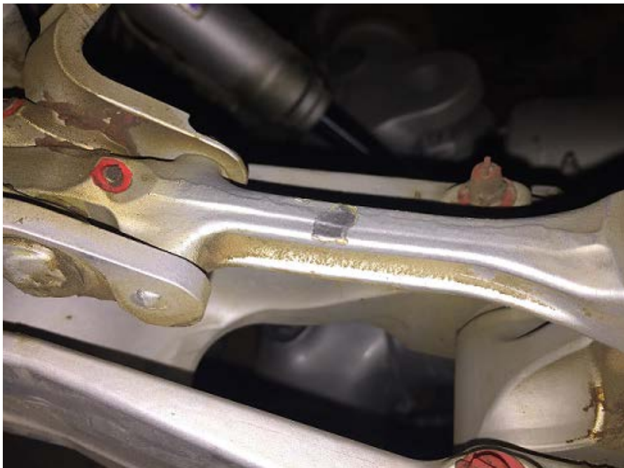
Damage to link caused by contact with collar
